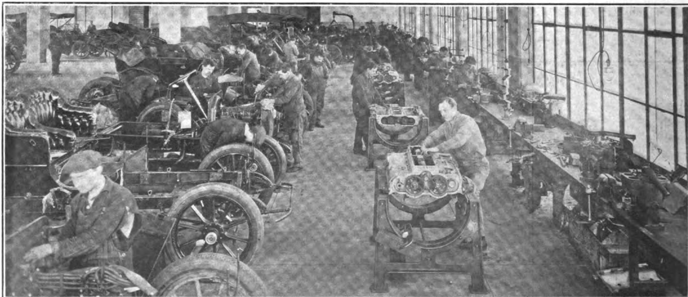
Fig. 7—The pleasure car repair shop. Men working on the motor are stationed nearest the windows to get the benefit of all the light possible
